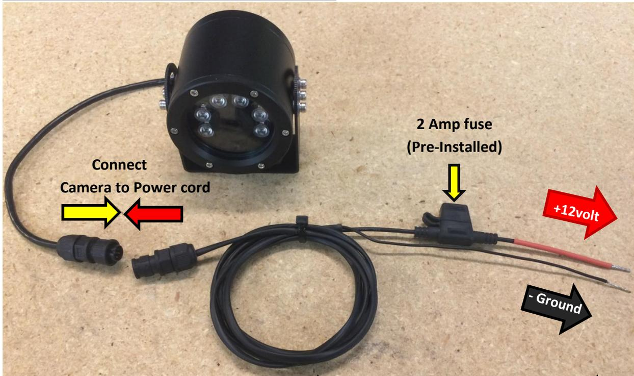
**Step 1:** Connect male 6-Pin connector (→) to the female 6-Pin connector (←) on the power cord.
