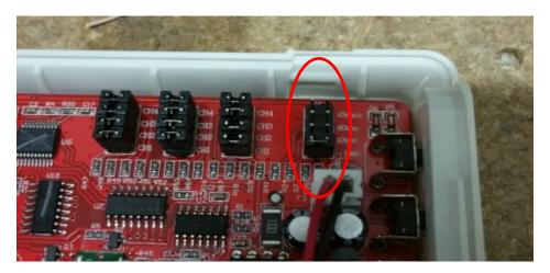
By default the siren is set to activate on all of the 4 zones. If you wish to change this setting, simply remove or add the jumpers in location "J1" on the receiver board. If there is no jumper present, that zone will not activate the siren. If the jumper is present, that zone will activate the siren.
