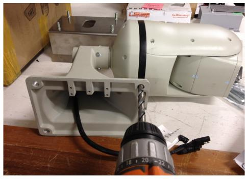
Mount the bracket on the pole or wall before installing the camera.
