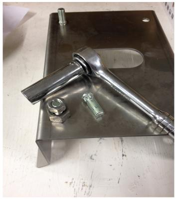
To install the Track bolts, use a 1/2"nut as a spacer, then pull the track bolt into the mount with the supplied 3/8"course flanged nuts.
