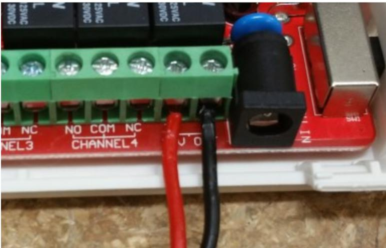
Now plug in the receiver using the black 12V 1A (or higher) power supply that came with the kit . Do not use the white 12V 500mA power supply that comes with the receiver as this one cannot supply enough power to run the siren.
