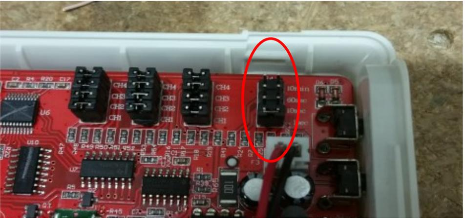
By default the siren is set to activate on all of the 4 zones. If you wish to change this setting, simply remove or add the jumpers in location “J1” on the receiver board. If there is no jumper present, that zone will not activate the siren. If the jumper is present, that zone will activate the siren.
