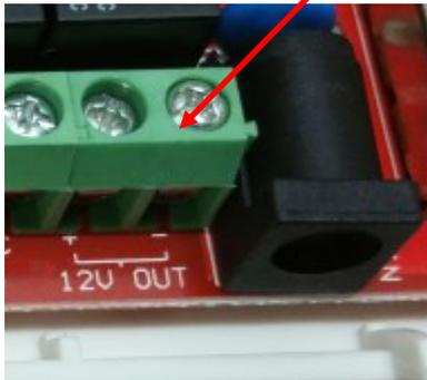
Using a small Phillips or flathead screwdriver, loosen the screw terminals.
