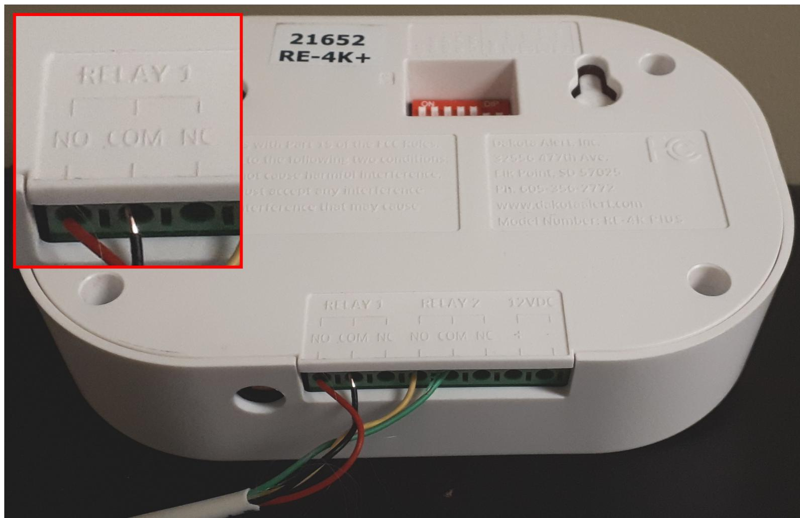
On Relay 1, the red wire goes to NO, and the black wire goes to COM. Follow the instructions that came with the receiver to properly connect the wires.
